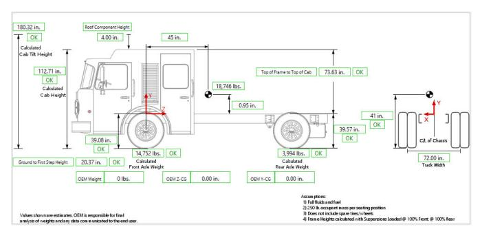
Calculated Apparatus Weight18,746 lbs.Calculated Apparatus Z-CG45 in.Calculated Apparatus Y-CG0.95 in.
